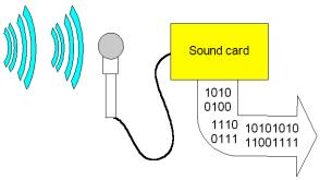
Take analog signals from analog sensor (e.g. microphone) and digitally sample data (More details later)
