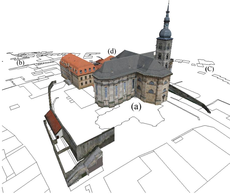
Figure 1: 3D scene registered with 2D ground plan data. Also illustrating how names of places from Web 2.0 sources can be integrated into the 3D model once they are associated to an underlying 2D ground plan. (a) St. Stephan (church), (b) Obere Pfarre (place of worship), (c) Klosterbrau (pub), (d) Battingerhaus (attraction), 3D model is shown positioned above the 2D ground plan for visualisation purposes.
