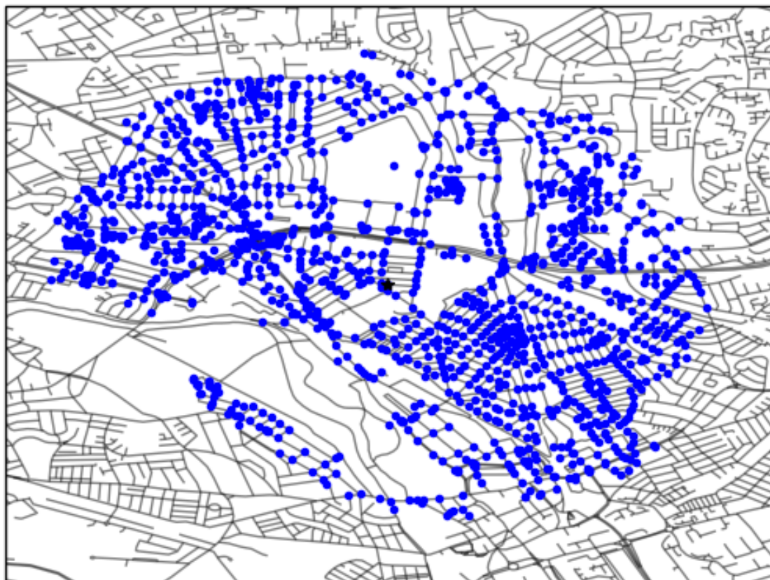
Figure 24 - Reachability Graph For Sample Node - Modified Dijkstra's
